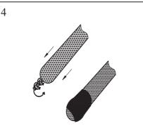
Pull back braid to cover the sleeve SCPC2. Twist the braid end and bend it. Position one heat-shrink sleeve SCPC1 as shown and shrink.
